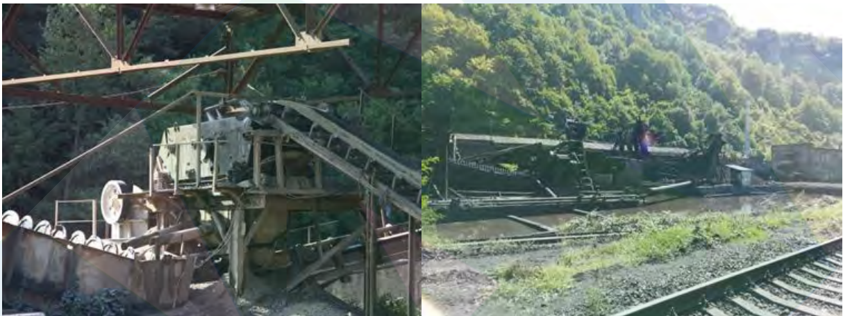
Figure 21: Mn ore processing technology – ore crusher Georgian Manganese (left), active ore crushed and tailing pond (right)
